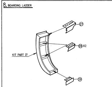
Replace plastic steps with etched brass items. Fold brass steps as shown. Two sets are included to do both sides of aircraft although starboard stairwell will need to be scratchbuilt. See Ted Taylors article in September 1989 issue of Scale Models International for further building hints and tips.
